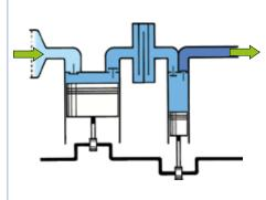
A multi-stage compressor has two or more cylinders connected in series in which air is gradually compressed to the final pressure.
