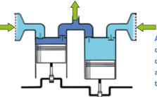
A one-stage compressor has one or more cylinders, each of which compresses air from atmospheric pressure to operational pressure.
